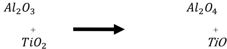
Illustration 3: Chemical reaction between pillar and aluminum oxide
