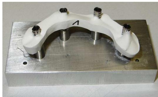
Picture 1 and 2: Measure between pillars and plaster key for Sheffield test
